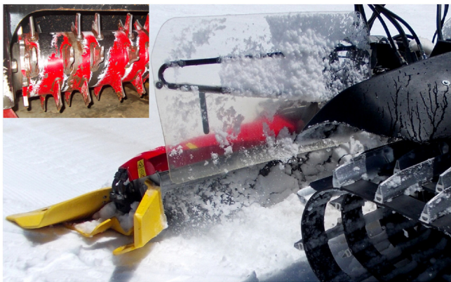
Fig. 3. The tiller is mounted at the rear of a grooming machine and consists of a high speed rotating shaft (cutter bar) with multiple tines which act as a mixer for the top of the snowpack.
